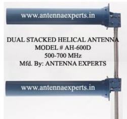
**BEAMWIDTH:** If the dual stacked helical antenna installed as per given configuration, the 60 degrees horizontal and 30 degrees vertical beam-width can be obtained. Similarly the dual array can be stacked horizontally to control the beam-width in horizontal plane without disturbing the vertical beam-width.
