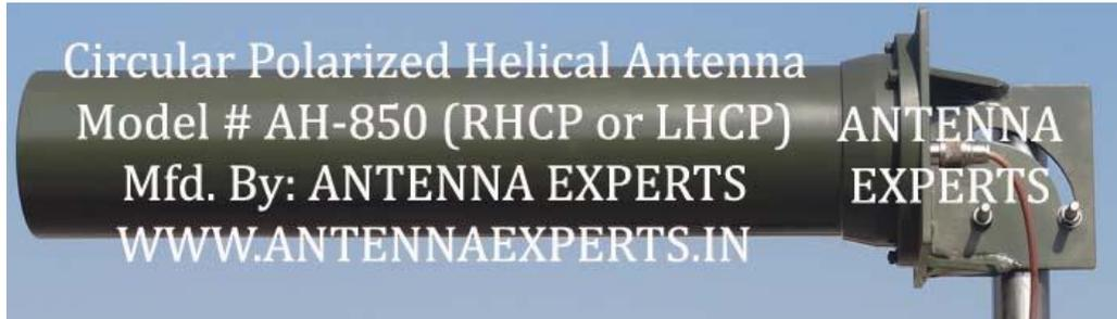
interference. Both Right Hand Circular Polarized (RHCP) and Left Hand Circular Polarized (LHCP) helical antenna models are available. The AH-850 Helical Antenna is light weight, broadband and rugged helical antennas, supplied with ABS radome to protect the antenna from environment. Cylindrical enclosure is used for low wind loading and for minimal effect of ice formation on the helical antenna operation as well as providing an aesthetically pleasing appearance.
