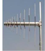
which is 0.75 meter. All elements are supplied in two segments for easy of shipping and handling. The elements are attached via a fast deployment self-locking device at points along the boom. The log periodic antenna operates at D.C. ground with low resistance discharge path for protection against lightning and immunity to noise. All the screws, nuts and bolts of log periodic dipole antenna are made of stainless steel.
